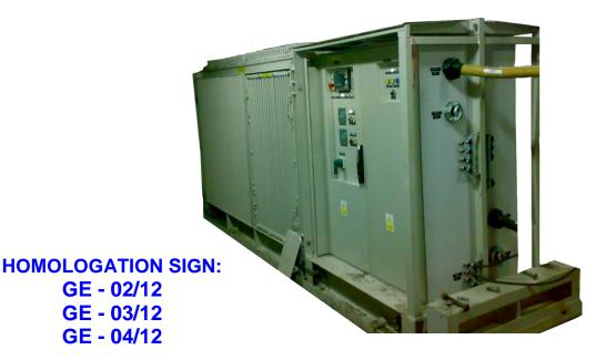
The transformer station type ST-T2/N1M1 is a device designed for use in underground mining in excavations with no explosion hazard or in conditions with no methane explosion hazard and designated as class A coal dust explosion hazard.
